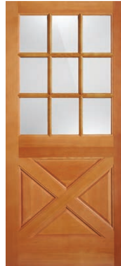
F2035 Single Pane Safety Glass 1-1/4" TDL Bar 3/4" Double Hip Raised Panel Ovolo Sticking 2/8 x 6/8 3/0 x 6/8
