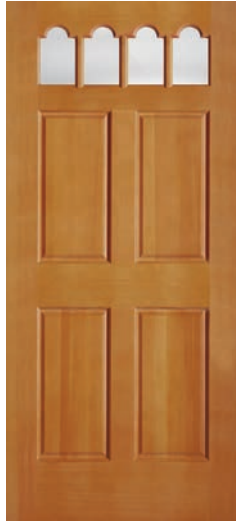
F2005 Single Pane Safety Glass 1-3/4" TDL Bar 3/4" Double Hip Raised Panel Ovolo Sticking 3/0 x 6/8
