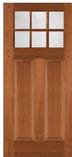
SM77662 Low-E 7/8" SDL Bar 1-7/16" Double Hip Raised Panel Ovolo Sticking Wide Layout 3/0 x 6/8
