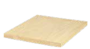
C-6971 Skirtboard 1" x 4" (ACTUAL 11/16" x 3-1/2") C-6973 Skirtboard 1" x 8" (actual 11/16" x 7-1/4") C-6975 Skirtboard 1" x 12" (actual 11/16" x 11-1/4") RO, MAPLE, WO
