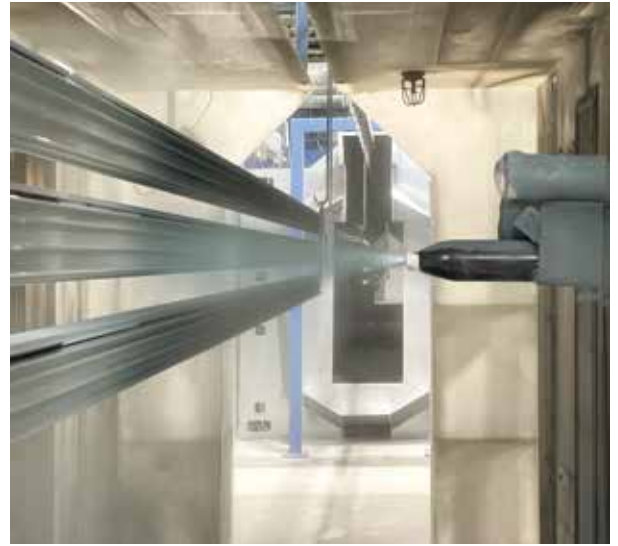
Steel blue powder coat finish being applied to our panel components.
